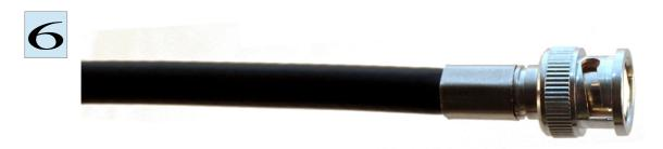
Crimp the crimp jacket with a crimp tool; herewith the copper braid will be trapped between the crimp jacket and the connector housing.
